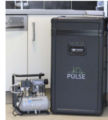
Equipment for a pulse airtightness test. The method is non-intrusive and typically takes under an hour to be applied (source: Build Test Solutions)
