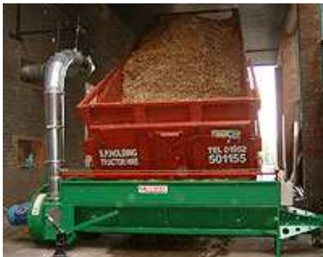
Trough fed wood chip blower used for delivery of fuel into an above ground silo. The fuel store can be 10-15m from the delivery point but blower is noisy and delivery slow, about 8 tonnes in 30 minutes.
