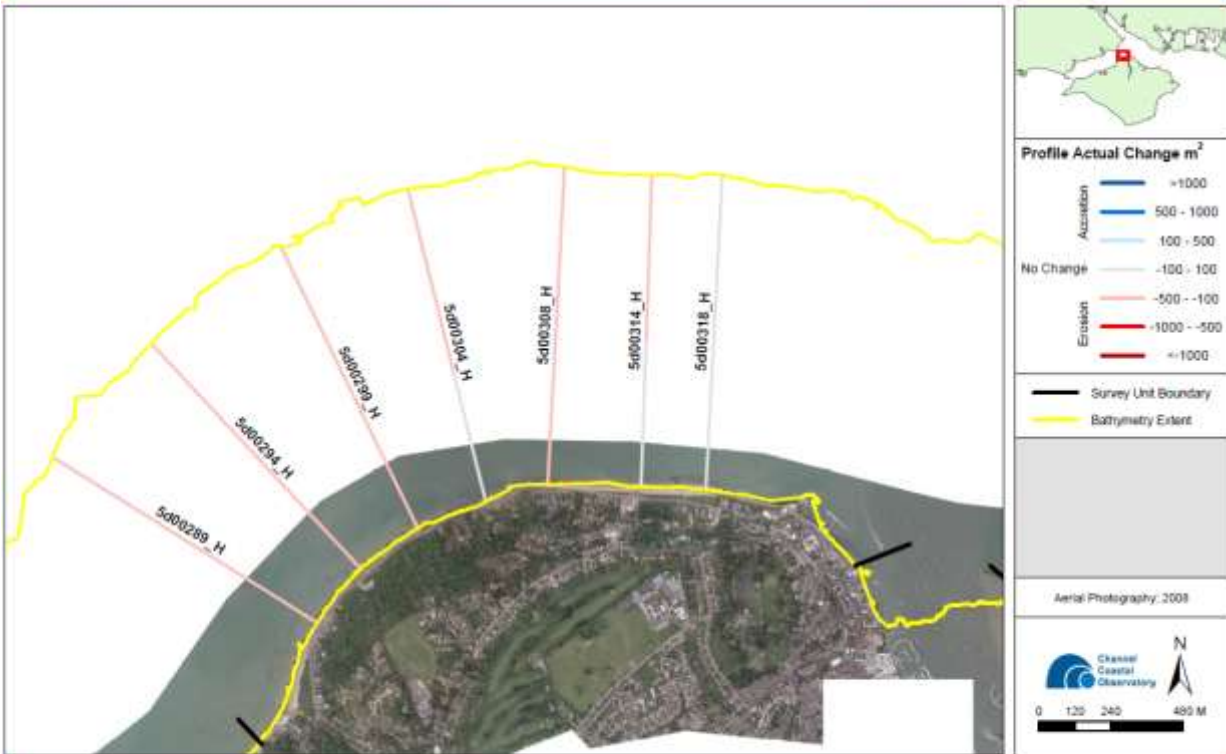
Bathymetry Profiles - Actual change in cross-sectional area 2006 to 2011 Gurnard Bay East to West Cowes: 5dSU12
