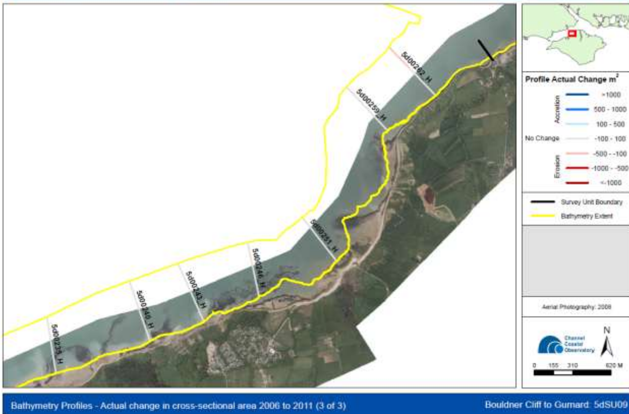
5-year change in the cross-sectional area of bathymetry profiles, Thorness Bay and Gurnard, from 2006-2011 (CCO, 2013)
