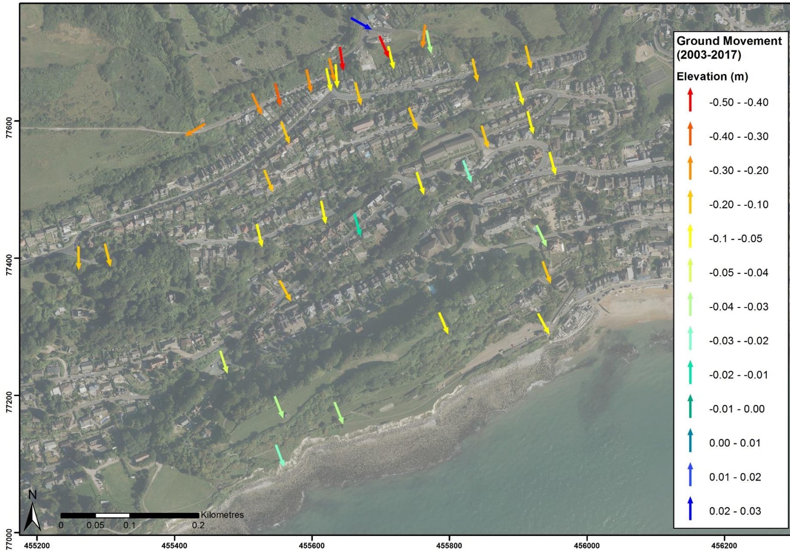
Figure 3. Ground surface elevation change at each of the permanent ground markers at Ventnor Park between 2003-2017.
