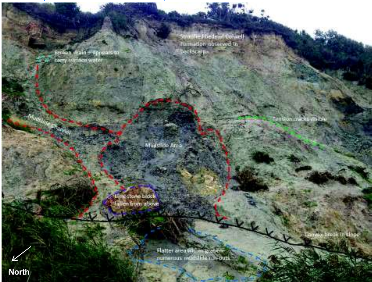
Figure 4.5: Recent Mudslides observed on the 22nd of October following a period of heavy rain. Image looking up at the Back scarp on the southern side of the landslide, within Section B.
