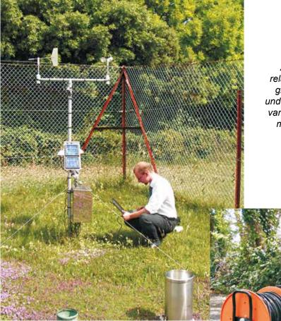
An improved understanding of the relationship between rainfall levels and ground movement can help assist in understanding landslide risk. Rainfall and various types of ground movements are monitored continuously by over 200 instruments within the Undercliff.
