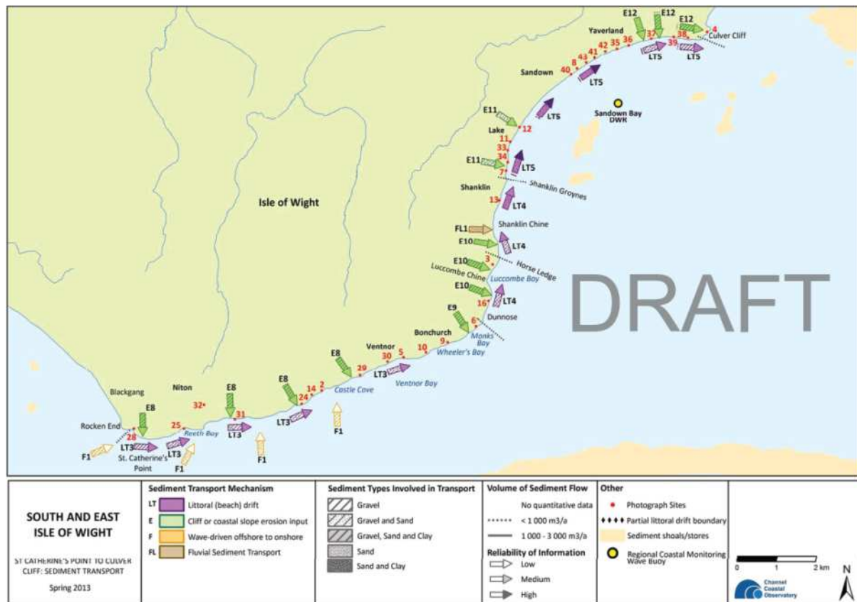
Figure 4-1. Sediment transport on the south east coast of the Isle of Wight, SCOPAC (2014, in press 2017)
