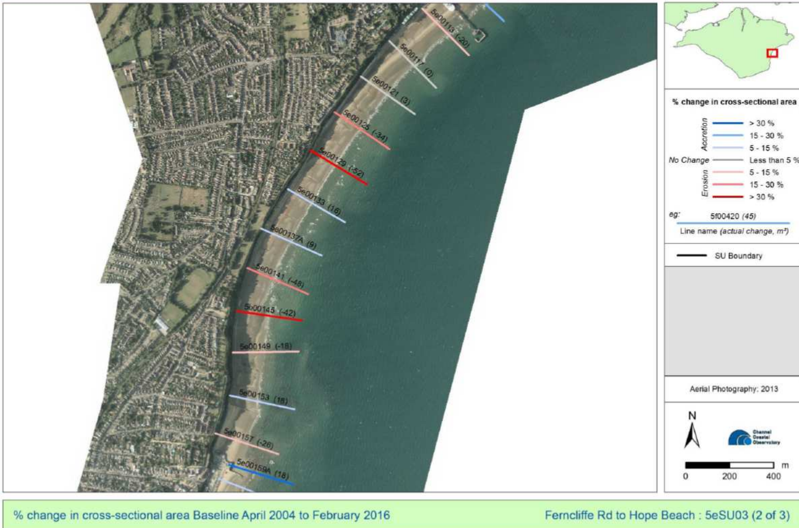
Figure 4-8. Beach profiles in the central section of the study site (obtained from the CCO, 2016)
