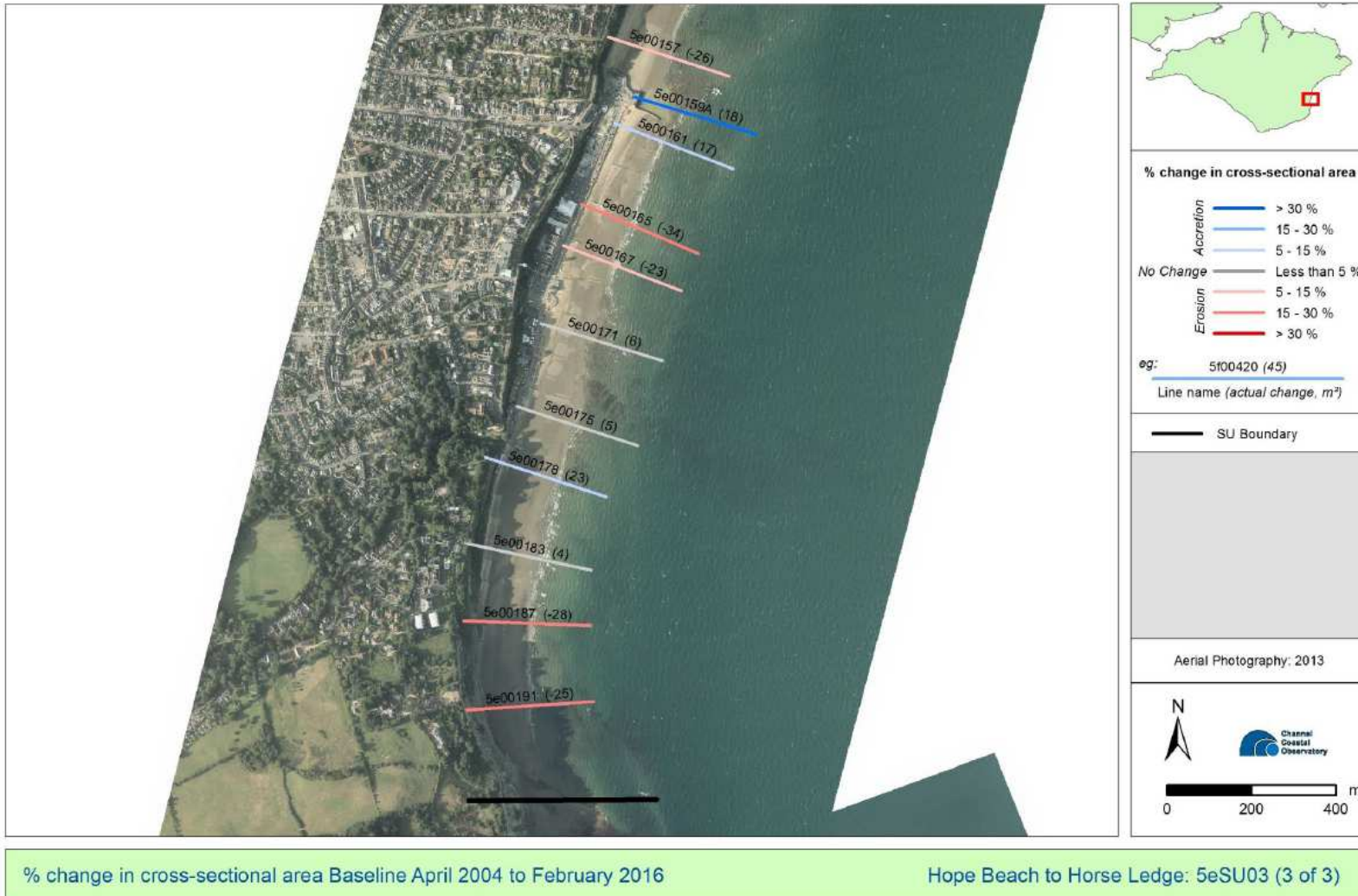
Figure 4-9. Beach profiles in the south section of the study site (obtained from the CCO, 2016)
