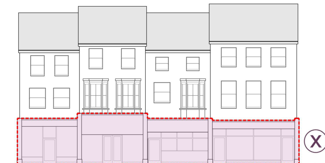
An example of a group of shopfronts with poorly designed proportions
