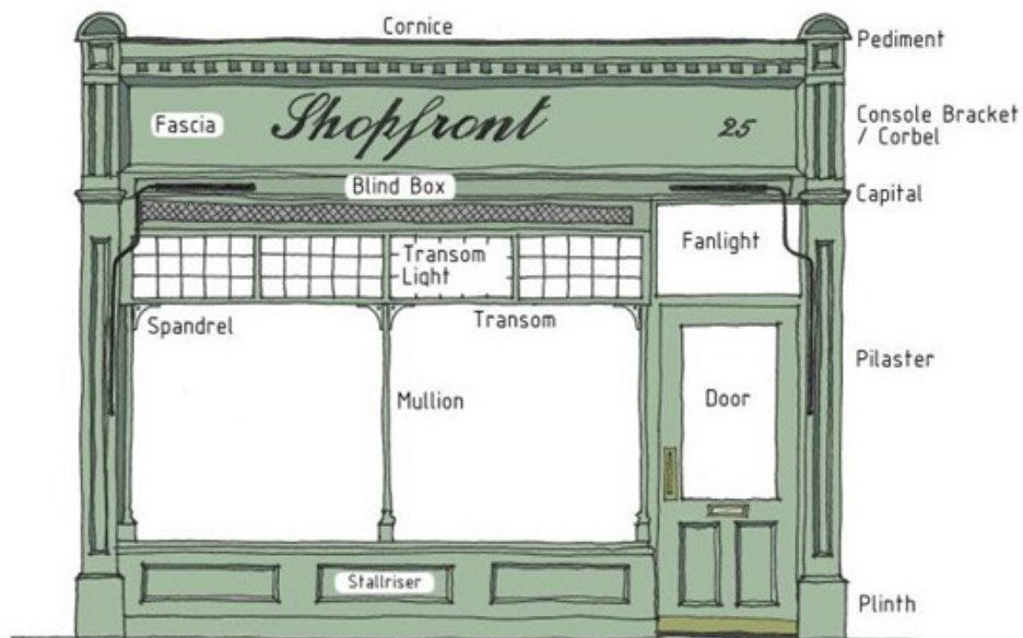
Typical traditional shopfront with architectural features labelled
