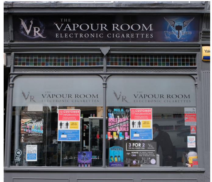
Coloured glass can be used in transom lights to conceal a low-false ceiling inside the shop
