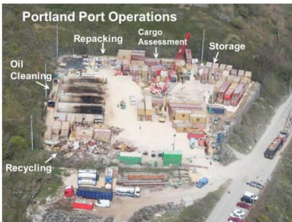
Figure 2 - The banded areas as set up during the NAPOLI operations at Portland Port in 2007 is an example of good practice.
