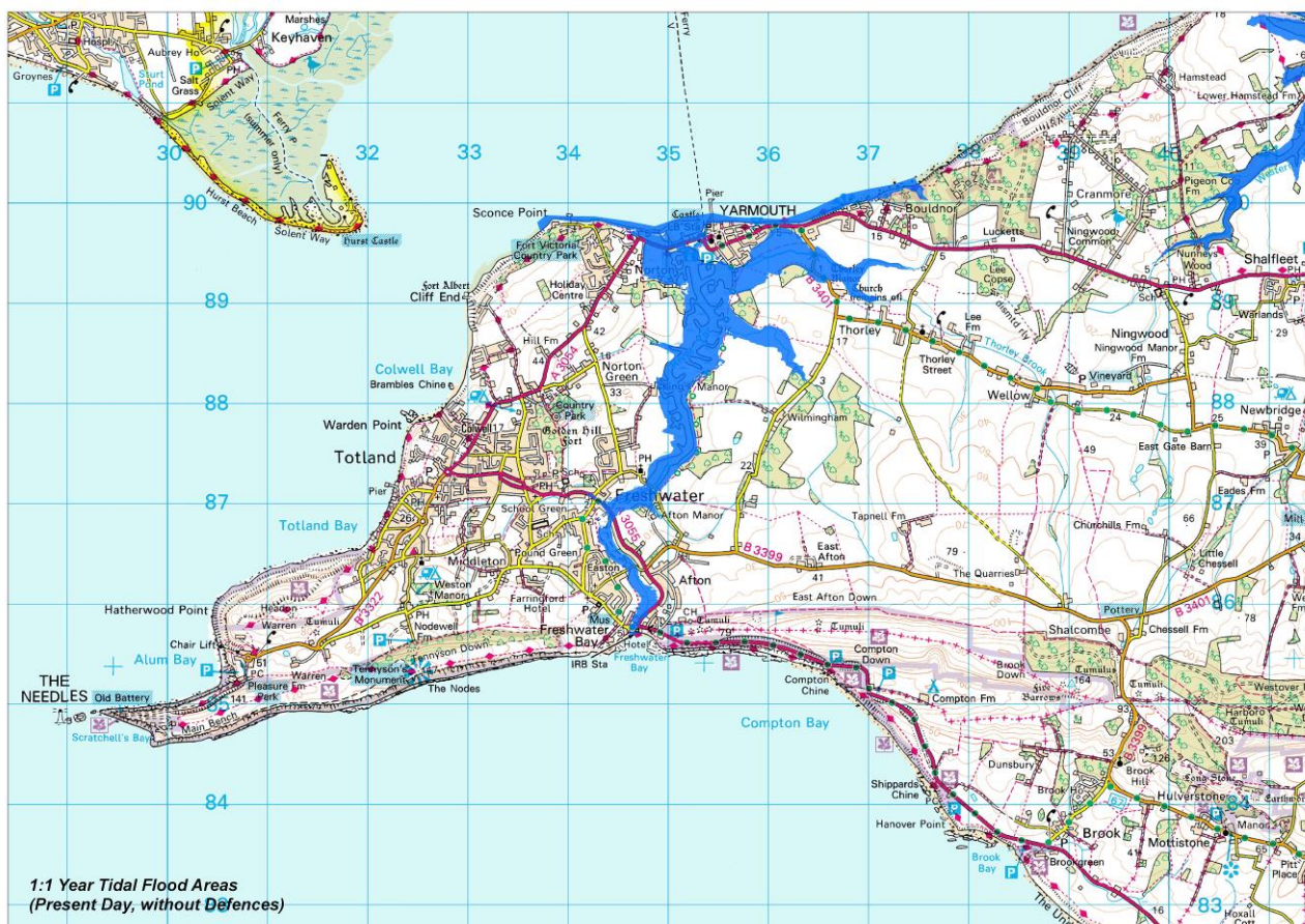
Current potential tidal flood risk in the Western Yar, if defences were not in place (1:1 year tidal flood area, present day). This image shows the low-lying nature of the valley and that current vulnerability to tidal inundation would already exist without the defences in place at Freshwater, Causeway Road and across Thorley Brook.
