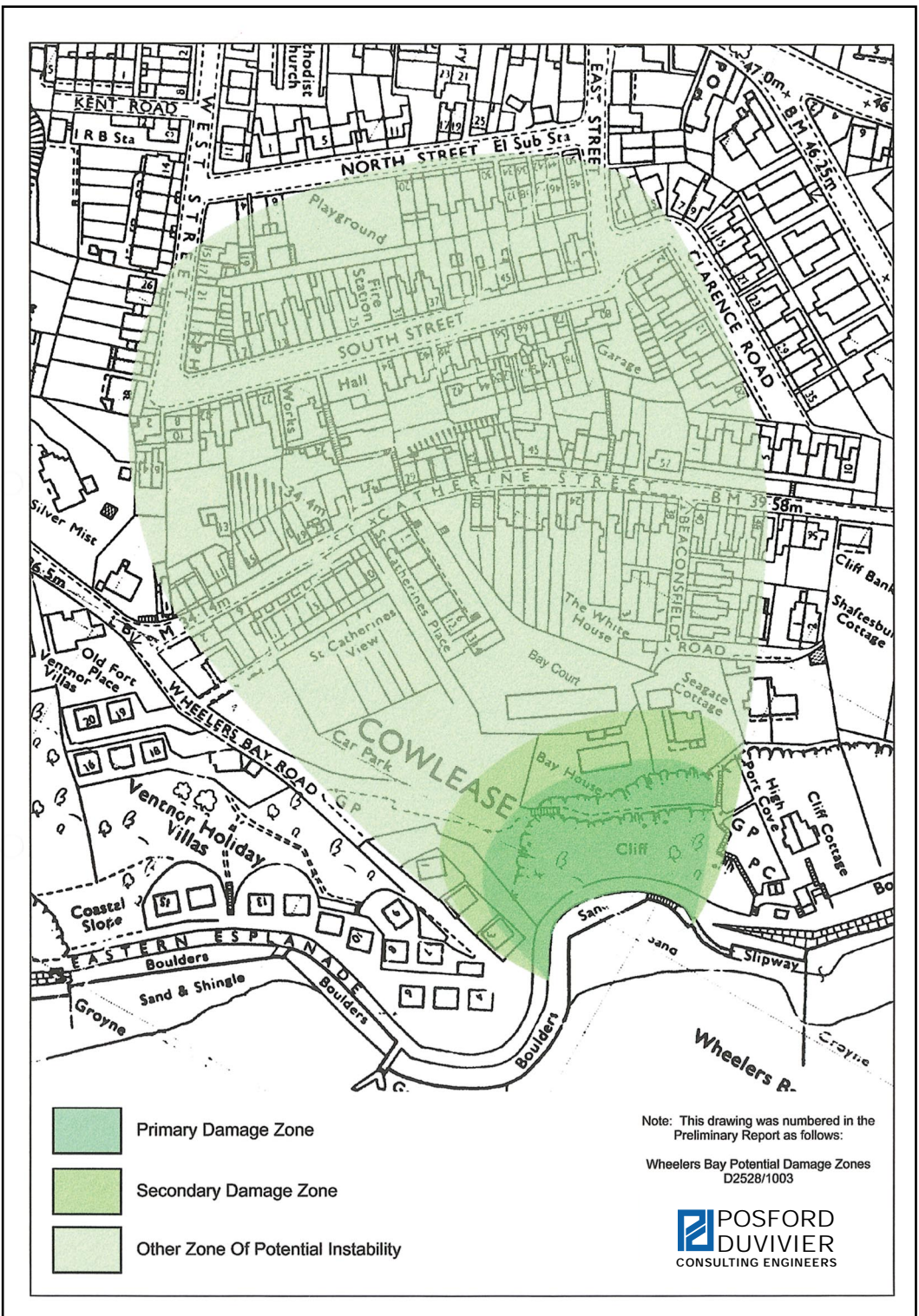
Figure G5.2 Landslide hazard map.
