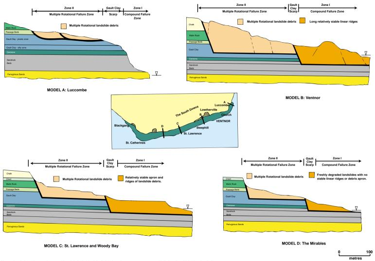
Note: Gault Clay Scarp obscured by debris in Models B-D; shearing may occur at multiple levels within the Gault Clay
