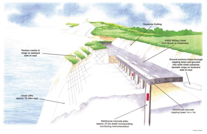
Figure G10.3 The proposed stabilization scheme.
