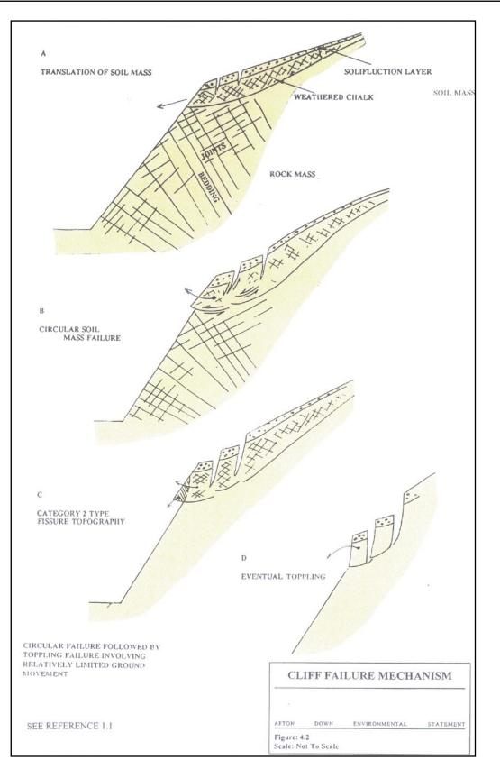
Figure G10.5 Cliff failure mechanisms.
