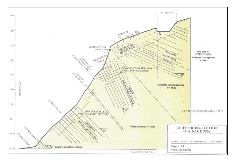
Figure G10.4 Cross section through the Afton Down cliff.
