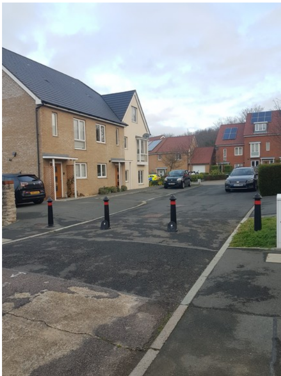
Figure 29: An existing modal filter in Oak Tree Way, East Cowes
