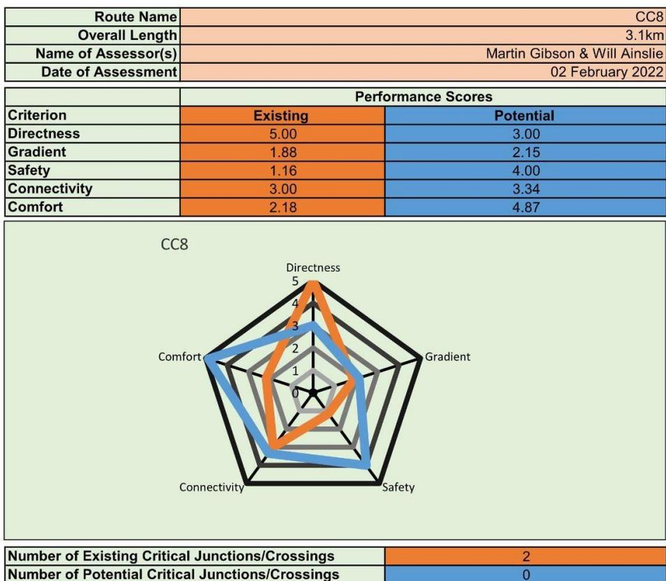
Figure 30 - Route Selection Tool output CC8
