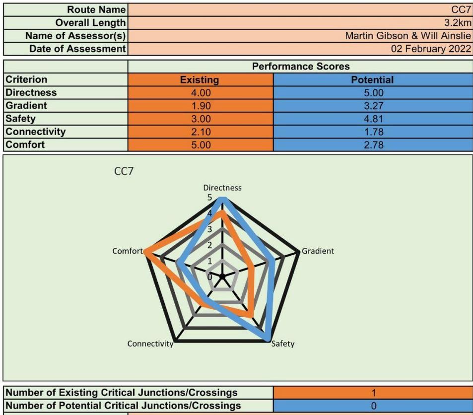
Figure 28 - Route Selection Tool output CC7
