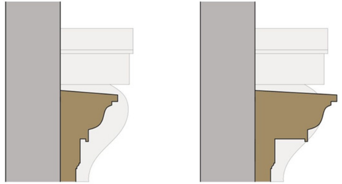
Ideal cornice overhang (L) contained within the extent of the console bracket.
