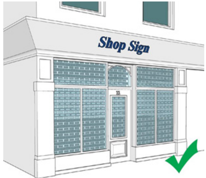
Security shutters should not be used externally, but instead behind internal lattice grilles, or preferably, laminated glass
