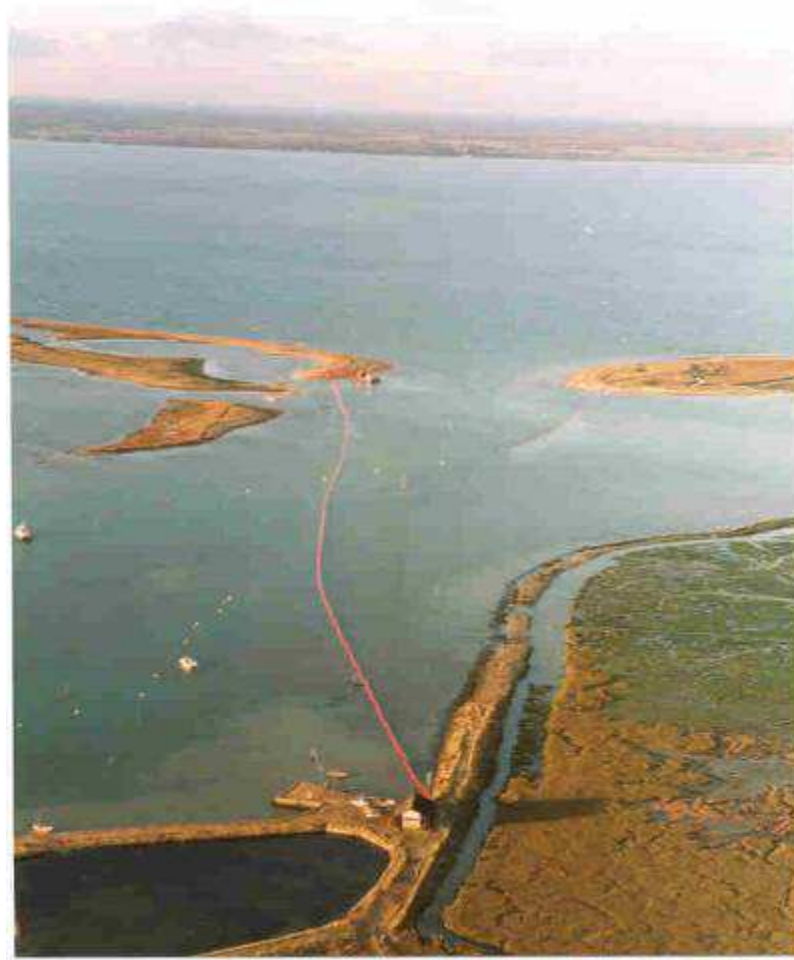
Fig 2: Newtown Creek Boom Deployment
