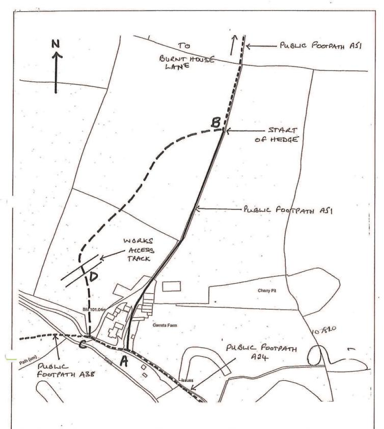
Part of A51 to be diverted during mineral workings then restored shown A-B (bold continuous line) Diversion route of A51 for period of mineral workings C-D-B (bold broken line) Continuation of N51 and other public footpaths (A38 and A24) shown with short dashed line
