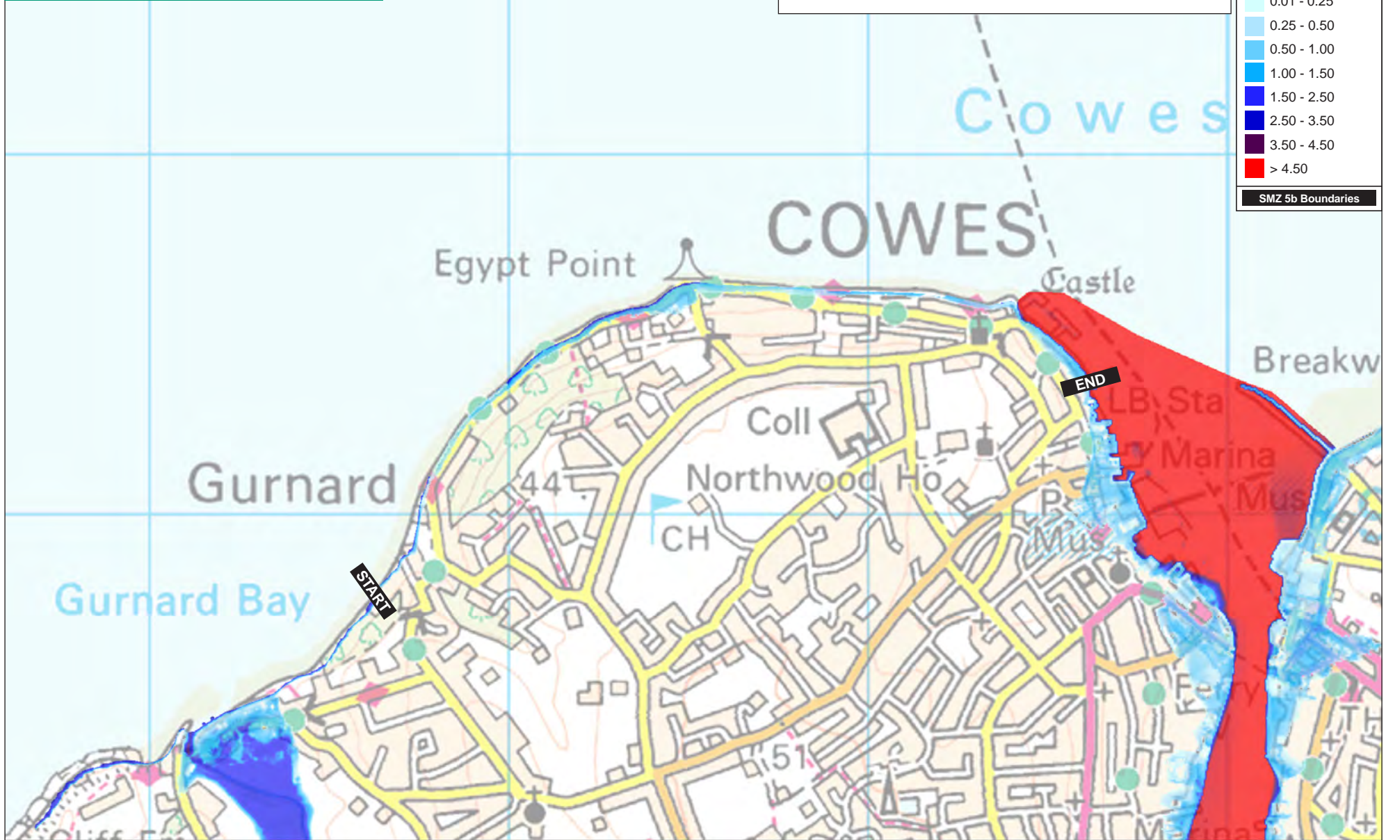
Maximum potential flood depths from a 1:200 year (0.5% annual chance) event with existing defences in place
